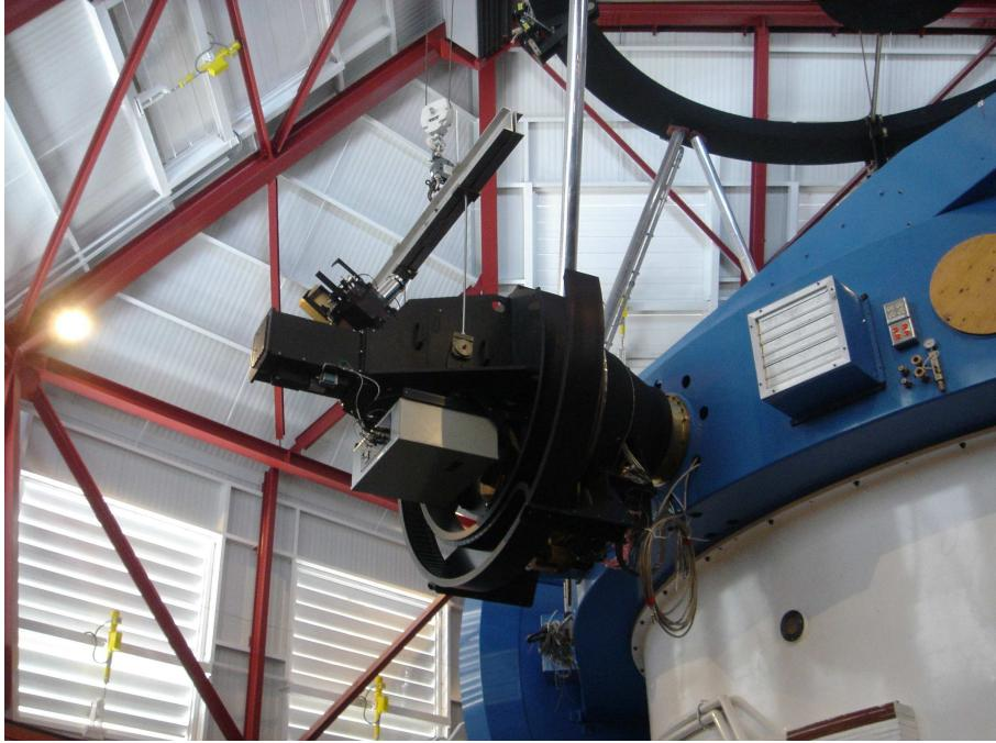
**Figure 1.** Photograph of MagE installed on the Clay folded port 2.
