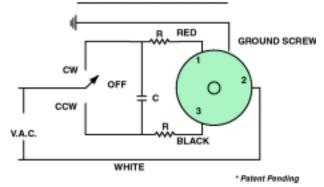
Number in diagrams represent terminal connection when motors are supplied with terminal boards.
